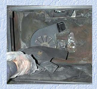
Remove the combustion blower cover plate and vacuum the fins of the combustion blower. An old toothbrush works well for removing deposits on the blower fins.
