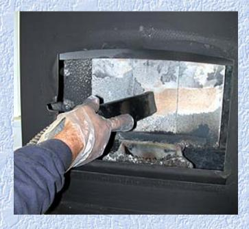
Using the pointed end of the scraper provided with your Harman stove and the vacuum, scrape the accordion heat exchanger and the surrounding areas free of all fly ash. Leave the ash pan in place and the ash door closed when cleaning the walls of the fire chamber. A 2" putty knife will help remove the ash. Holding the hose of the vacuum just below the where you are scraping helps to remove airborne dust and catch the soot as it removed.
